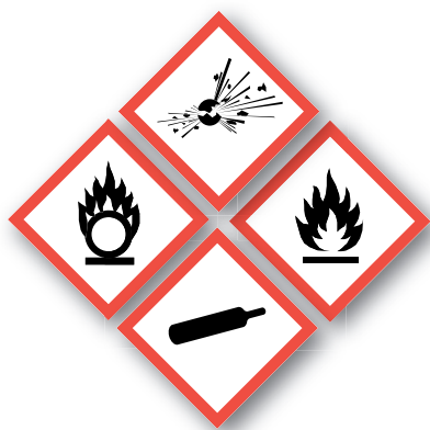
Sustancias explosivas e inflamables Explosive and flammable substances
